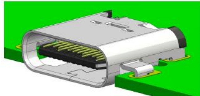
Figure 3-7 Reference Footprint for a USB Type-C Mid-Mount Dual-Row SMT Receptacle (Informative)
