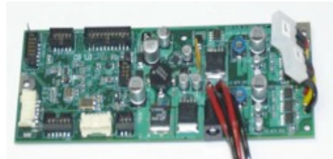
Reduced size with integrated processor, motor controllers and sensor interfaces
