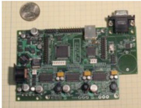
Integrated processor and motor controllers
